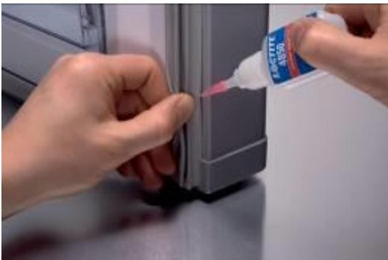
Fig. 2: For parts subjected to repeated flexing there are specially designed flexible cyanoacrylate adhesives, which can be used to attach rubber profiles to refrigerator doors or for similar applications.
