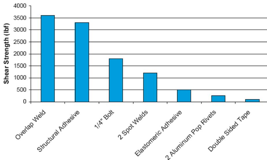
As shown in this figure, overlap welds and structural adhesives are the strongest assembly methods available. Strength drops off dramatically using bolts, spot welds, flexible adhesives, pop rivets and double-sided adhesive tape. For some applications double-sided tape may provide adequate strength, but for all applications a blend of adequate strength and lowest overall cost is the target.
