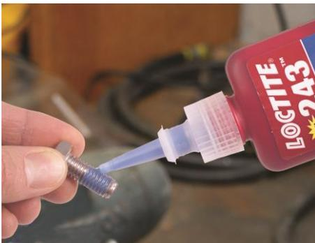
Threaded fasteners continually receive various types of differential stress. Stresses such as vibration and shock, thermal expansion and contraction, and micro-movement of the fastened parts all can reduce clamping force and, ultimately, cause machine failure. Many mechanical devices such as spring washers, wire retainers and locking bolts were created in an effort to prevent uncontrolled fastener loosening.
