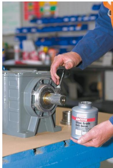
excess of 1,000 degrees and some perform in temperature extremes up to 2,400 degrees. Anti-seize can be used on a furnace door hinge, for example, preventing the hinge from seizing in the harsh environment.
