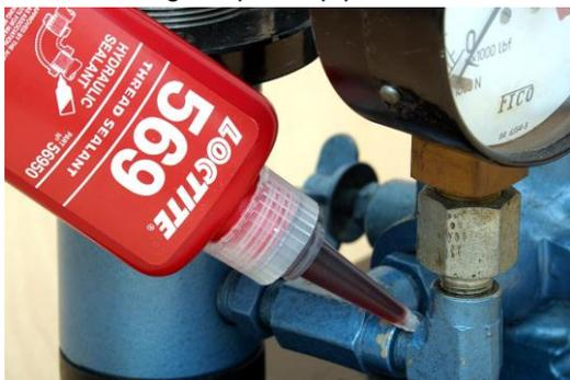
use and repair, the threads can become damaged and even more vulnerable to leakage. The area where the crest and the root of the thread meet forms a spiral leak path. No amount of tightening will eliminate this. Thread sealing is an attempt to block this leak path in pipe connections. Mechanical thread sealants include a variety
