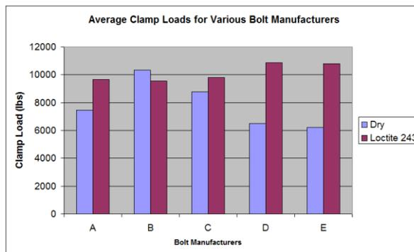
Graph 2 – Bolt clamp load variance with chemical threadlocker
