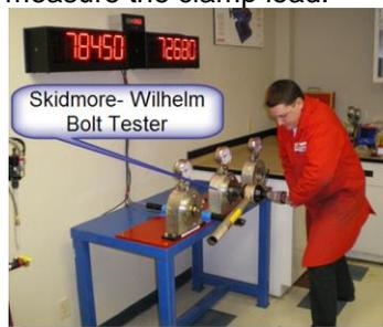
Picture 4: Torquing of bolts in load tester
