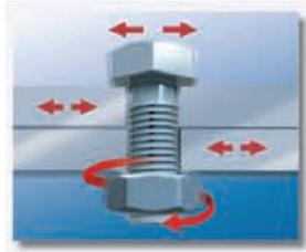
Picture 2: Vibration induced motion of bolted system
