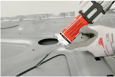
source of faults in practical application. Another essential condition is correct application of the adhesive by the staff. The effectiveness of bonded structures is heavily dependent on the production conditions. These include preparation of the fitted parts, correct mixing in the case of 2-component adhesives and their application as well as fixing
