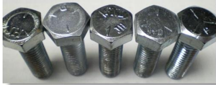
Figure 1 - Identically specified bolts from five manufacturers
